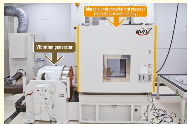
We completed the vibration testing facility at Kyoto Techno Center in June 2014. It is combined with the environmental test chamber by which the vibration test can be conducted both vertically and horizontally under the harsh environments to cover the temperature -40°C to +140°C and the humidity 20% to 90% RH.
