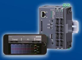
DL8 Series use the smartphone for the display and transmit data measured at worksite via wireless LAN or internet.
