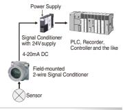
Field-mounted 2-wire Signal Conditioners **B6-UNIT Series**
