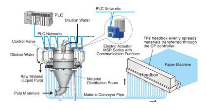
**Open Network Capable Linear / Rotary Motion Electric Actuators MSP/ MRP Series**
