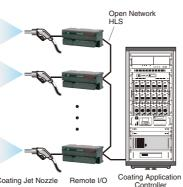
Coating Jet Nozzle Remote I/O
