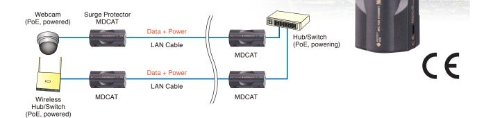
M-System's model MDCAT is specifically designed to protect communication devices connected via Ethernet LAN from lightning surge entering through network cables.
