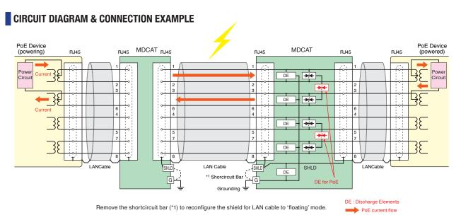
The above diagram shows the PoE Alternative A configuration example. The terminals 4-5 and 7-8 are used to supply power with Alternative B configuration.
